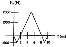
4. A 3.0 kg particle moving along the negative x-axis with a speed of 2m/s experiences the force shown. What is its speed and direction after the force ends? (-0.67 m/s)
