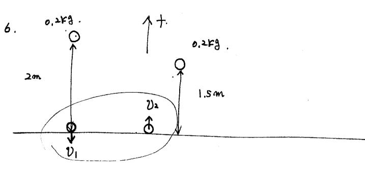
$$\Delta m v = 0.2 \cdot v_2 - 0.2(-v_1) = F \cdot \Delta t$$
