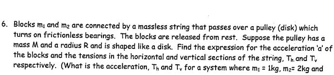
pulley has a mass of 0.5kg and radius 0.1m). ( $a = \frac{m_1 g}{\frac{1}{2} M + m_2 + m_1}$ , a=3.08 m/s², T<sub>h</sub>=6.15 N, T<sub>v</sub>=6.92 N)
