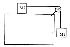
7. In an Atwoods machine setup, the two hanging masses are 4kg and 2kg respectively. The pulley shaped like a disk is 6cm in radius and has a mass of 2kg. As the pulley turns, friction at the axle exerts a torque of 0.5Nm. If the blocks are released from rest with the 4kg block 1m from the floor, how long does it take the 4kg block to reach the floor? (1.09 s)
